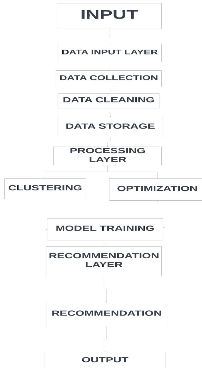
Figure 1: System Architecture for Recommender System
