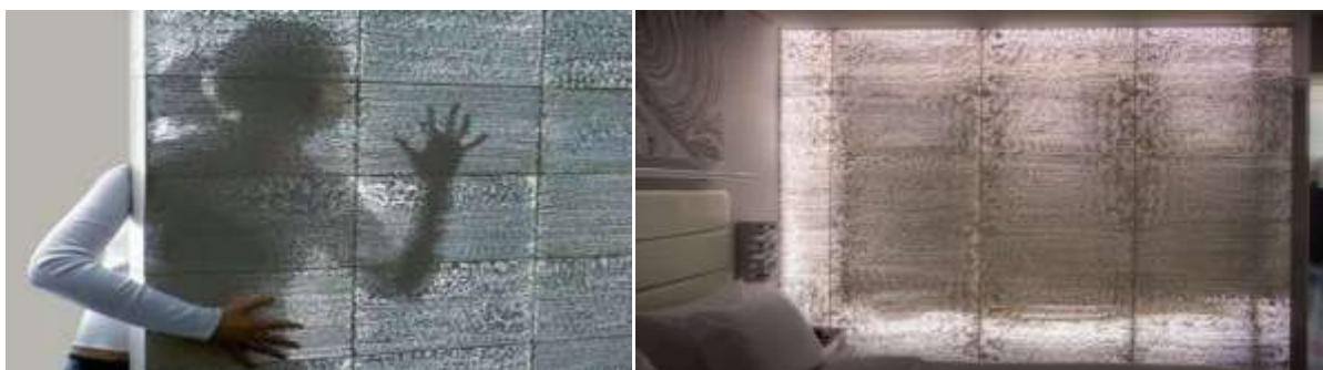
Figure 7.1 and 7.2; Aesthetic attractive interior view provided by using translucent concrete panels.
